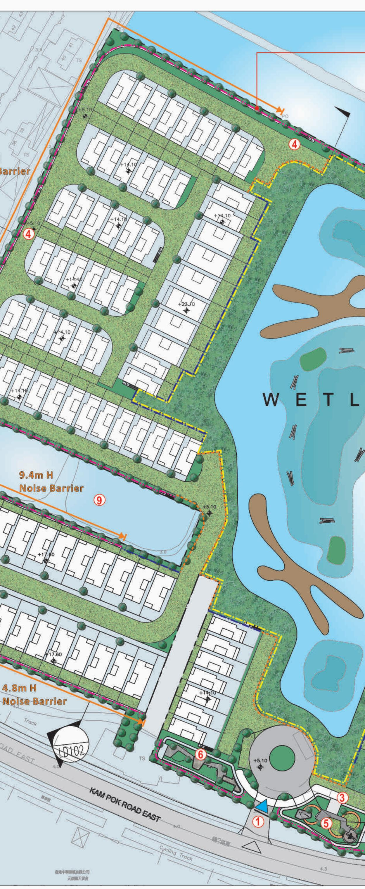
Noise Barriers composed of 2.5m H Solid Wall at base and **Transparent Panels on top to** minimize the visual intrusion of the Wall. Ornamental Trees, Shrubs, and Vertical Green Walls to provide Smooth Transition **Between the Development and** the Surrounding
